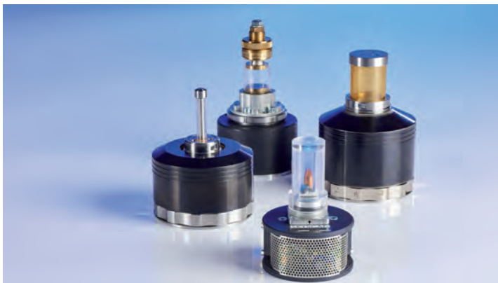
Non-ambient (up to +85°C, down to 40°C below ambient) and mechanical stages (up to 4400 N) for time-resolved 3D microscopy
