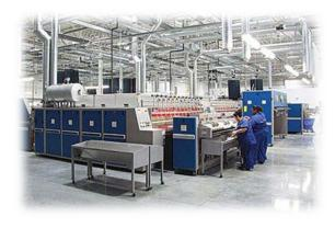
Three Chicago® flatwork ironing lines each include an Edge Maxx corner less spreader-feeder, FasTrak spreader-feeder and a Rapid Feed with vacuum for small-piece feeding. Sheets and small-piece goods are automatically processed through three 2-roll, 52-inch Powerhouse self-contained gas-heated ironers. Sheets are folded, stacked and delivered to a main conveyor through two Skyline automatic folders, and small pieces are folded and automatically stacked on a Skyline SP-4 ready for
