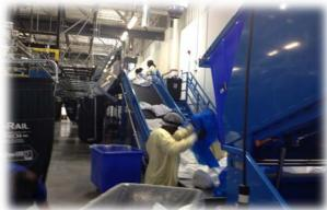
The Laundry Division of ARCO/Murray retrofitted the existing warehouse building to accommodate new Milnor washroom equipment, Chicago Dryer Co. finishing equipment, and E-Tech soil and clean rail systems, all provided and installed by Miami-based distributor Steiner Atlantic.
