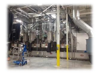
Adequate rail space is provided to accommodate 21,000 pounds of clean linen storage, folder, and hand-folding station. The clean-side storage system includes 70 slings and trolleys at 300 pounds capacity each.
