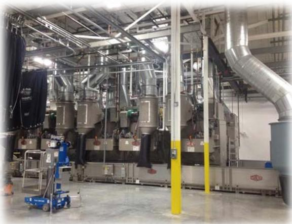
Adequate rail space is provided to accommodate 21,000 pounds of clean linen storage, folder, and hand-folding station. The clean-side storage system includes 70 slings and trolleys at 300 pounds capacity each.
